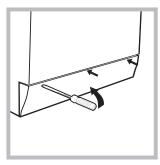
3. using a screwdriver, remove the cover panel on the lower front part of the washing machine (see figure).
