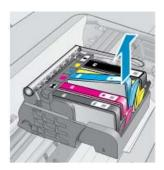
4. Lift the latch handle on the print carriage until it stops.
