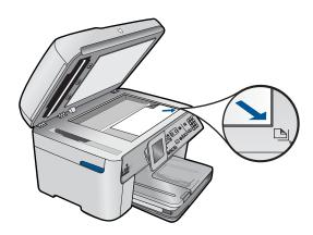
**Cause:** The original was not loaded or was loaded incorrectly.
