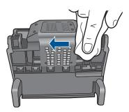
c. Use a fresh, lightly dampened, lint-free cloth to wipe the plastic ramps on both sides of the nozzles. Wipe away from the nozzles.
