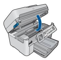
**Cause:** The printhead or ink cartridges were not installed or incorrectly installed. If this did not solve the issue, try the next solution.
