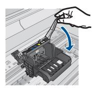
**Cause:** The print carriage latch was not closed properly.
