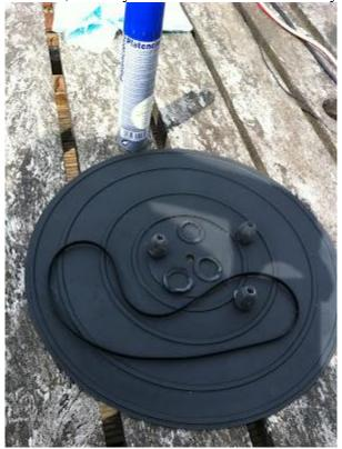
In a separate blog I restored a turntable mat from dull grey and hard to black and supple using Platanclene Printer Roller restorer. Again here I put all the smaller pieces in a plastic sandwich bag along with a few squirts of Platanclene, then worked the fluid into all the rubber parts, especially the bushes around where they slot into the motor top plate.
