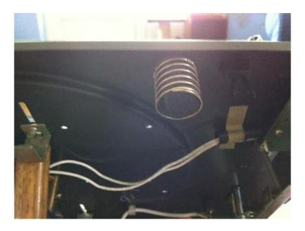
I cut 4 wads of foam, roughly the size and shape of the space inside the springs, and stuffed these into each of the four main springs as you see. Once this is done and the top lowered back into place, the deck looses the unmanageable springiness. The suspension is stiffer and slower, with less bounciness.
