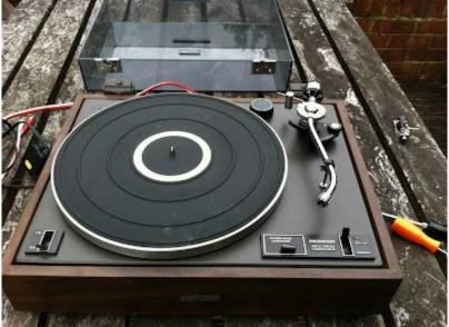
I then carefully lifted off the mat which should come away from the spindle in the middle. It has a decorative metal hoop which sits in a trough in the mat,
