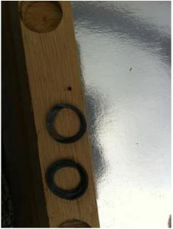
Of the 4 wooden recesses in the base for the springs, two had rubber washers in. On closer inspection one had two such rubber washers in, so I had 3 washers in total. These may be to provide further decoupling, but I think it more likely they are to balance the top plate i.e act as tiny shims. I removed these and put them carefully to one side.
