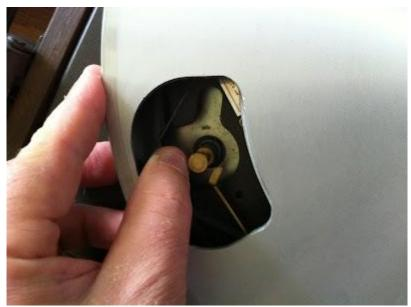
Now you can see the platter, and a couple of holes either side, if you rotate the platter you will see where the motor spindle has the belt looped around it beneath the platter. If you slip the belt off the motor through the hole you should be able to lift the platter off, a gentle vertical lift.
