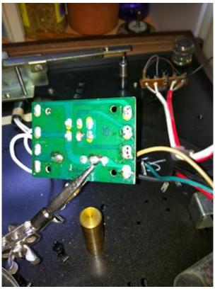
Here it's useful to use a craft stand / clamp to hold the board as you need to operate both a soldering iron and de-solder device applied to each of the 4 solder pads. in the picture above you can see a number of tabs removed. This is a gentle slow process, removing as much of the solder from each tab base as possible , then gently working loose while applying heat with the iron. Eventually I got all 4 loose and disconnected the motor from the top plate via the 3 bolts.
