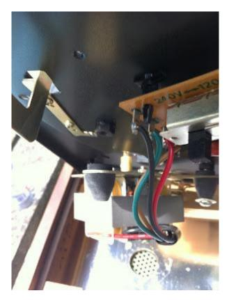
Here you can see the motor with one rod removed, free from the top of the plinth
