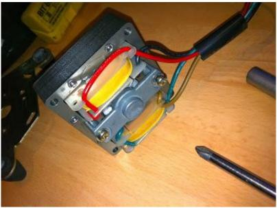
The motor frame is held together with two bolts. These are secured by two bolts and two further nuts (now removed) held the mounting plate to the motor.
