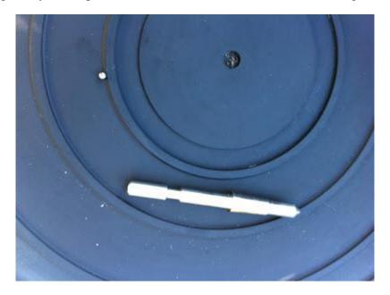
While warm soapy water got rid of some of the grease, it didn't get rid of all of it. I used Servisol Switch cleaning and some rubbing with a soft cloth to clean the spindle shaft to shining. I used the same liquid and a dozen cotton wool buds to clean the inside of the brass well until the buds were coming out clean and not yellow from grease or grey from steel filings.
