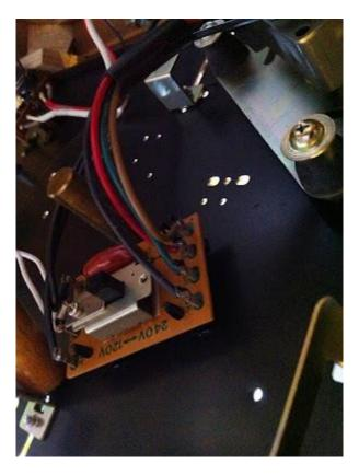
You can see the motor on its 3 rubber mounts. From the motor are 4 coloured wires which connect to a small circuit board. This board has a switch which is secured in position by a metal plate. This is to select between two voltages 120v and 240 v AC.
