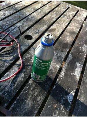
I use Chain saw oil, which is a little thicker, but most synthetic oils will work. Some favour sewing machine oil. Once the spindle is back in and settled, I tightened the retaining
