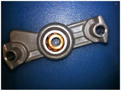
Here is the underside of the upper bearing frame with the bronze collar bearing clearly visible
