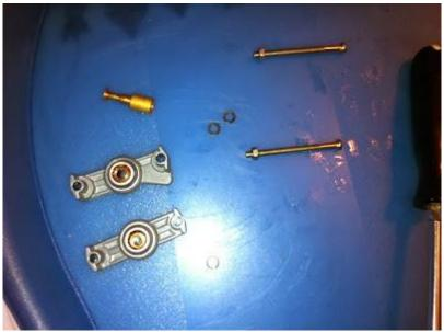
Above you can see the two bolts, nuts and split washers, the brass 45/33 motor spindle AND the upper and lower bearing frames. These last two were the focus of my work.
