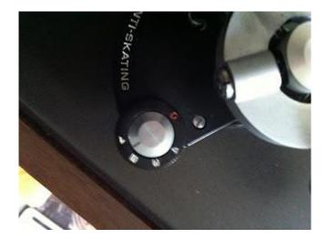
Once the tracking weight is set you are almost done. There are three remaining settings. First bias aka Anti-skate. On the Pioneer and many other decks this is set via a small wheel and is set to the same value as the tracking weight i.e 1.75 for me. This function compensates for the effect that inertia has on the arm, where the stylus will have greater pressure on the outside groove wall than the inside.
