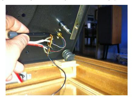
I gently slackened the side screw with a very small jewellers screw drive (cross head). I found that I could then very gently tighten the brass collar with my finger tips, as one would tighten a nut. I did this only just finger tight as too tight would create too much pressure and friction on the bearing. Using the side screw position as a reference I found that if the screw pointed to 9 on an imaginary clock face, then I could tighten it to 10 or 11, without applying any undue force.
