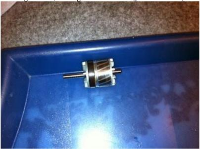
Here is the central rotor part. Both the rotor and stator were clean and the only treatment I gave the rotor was to wipe the two steel rod ends with a clean cloth.
