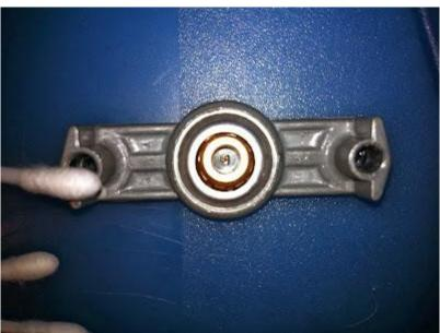
Here you can see the inside of the lower bearing. There is a bronze internal bearing into which the motor spindle sits . In the very centre you can see a mark which a wipe with a cotton bud removed. It appeared to be some black dirt in the bearing well, possibly original grease mixed with worn metal.
