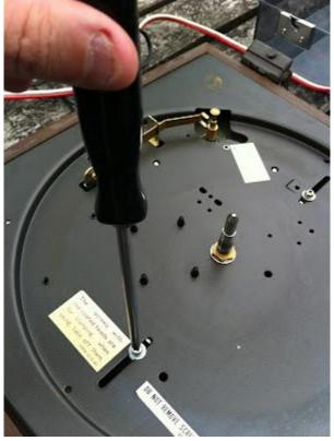
Once these are slid to the centre the deck top should be able to be tipped up. Some care is needed as the cables are captive at the back and the 4 springs are still engaged in their 4 circular recesses, but I find holding the speed selector and on/off switches on the top, I can
