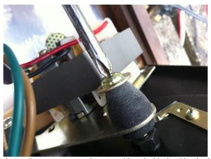
In the inverted picture above you can see the motor. Note the black rubber bushes, which the motor sits on via the three threaded rods.
