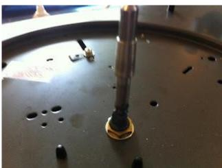
Two more drops into the motor. I then removed the spindle again, cleaned off the oil and tried a thicker Castrol Moly Grease, in case the noise was some scraping in the main bearing. I've used this grease before where I appeared to have some play in a bearing and it seemed to work well. It contains Molybdenum Disulphide.
