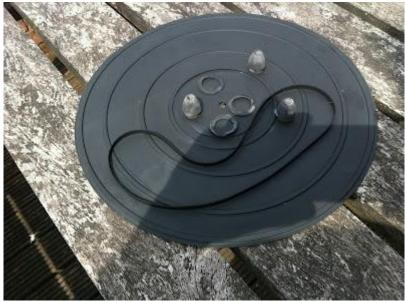
Now all the rubber bits I extracted, I put together including: the matt, the belt, the 3 washers at the base of the springs, the three bushes that support the motor. I should have included the 4 feet which screw into the base, but they looked OK and do not really need the next process.
