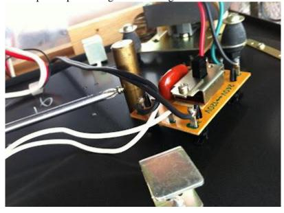
This inverted picture shows me loosening the screw. It doesn't need to be completely extracted. Eventually it will be out sufficient to allow the spindle to be extracted. Once I had removed the spindle, on inspection there was a lot of brown hardened grease on the shaft. I placed the spindle in some hot soapy water to gently remove the worst.
