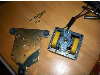
Then remove the top mounting plate from the motor. This is held on by two nuts and split washers. I also remove the brass 45/33 RPM spindle which is held on by a small grub screw. Keep these and all other parts safe, I tend to use a plastic tea tray to store stuff on.
