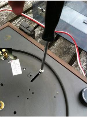
Gaining access to the underneath of the deck is very easy. Two screws on the top are slackened and you can then slide the screws and the brackets they connect with toward the centre of the deck. You are sliding two clamps from the wooden internal ledges they
