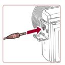
Open the cover and connect the external microphone.
